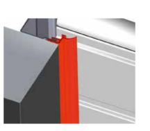
The seal lips on the lateral abutment
