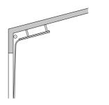
HLD: High lift guide rail fitting following roof line (max. 30°)
